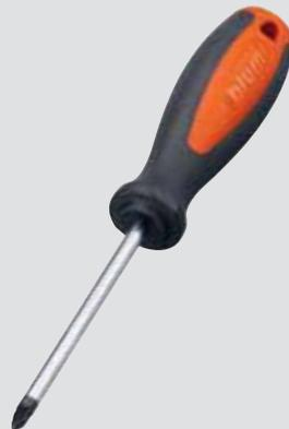
A POZI screwdriver (different from Phillips) is the most crucial tool you can use to assure that full torque is applied to all Blum mounting screws. POZI screws can be identified by the distinctive "tick" marks located in the center of the screw head recess.
